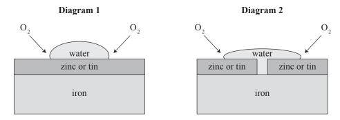
However, if the protective surface coating is damaged, as in Diagram 2, corrosion of the iron may still be prevented, if a suitable metal is in contact with the iron, by a process called cathodic protection.
